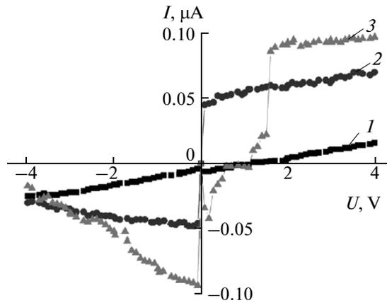
**Fig. 3.** Current-voltage characteristics of  $n$ -InP<Te> structure with simple ohmic contacts measured in the temperature range of 30–250°C at (1) 25, (2) 100, and (3) 150°C.
