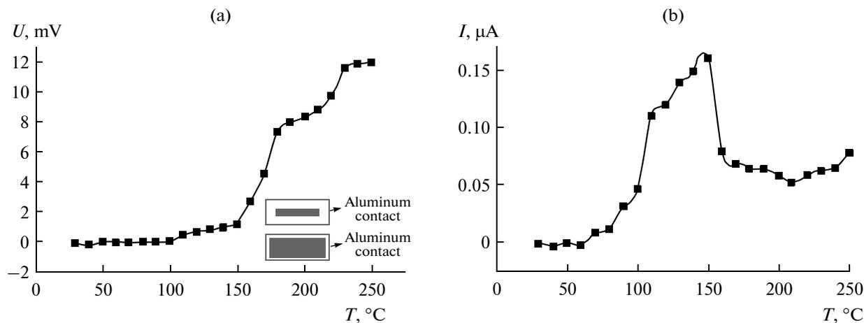
**Fig. 1.** Temperature dependences of (a) voltage and (b) current for  $n$ -type InP<Te> sample with ohmic contacts (schematic representation of sample is given in Fig. 1a).
