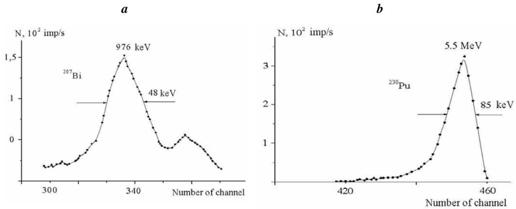
**Fig. 3.** The amplitude spectra of Si(Li)  $p-i-n$ -detectors with a large area of the sensitive area ( $\varnothing i = 110 \text{ mm}$ ,  $W = 4 \text{ mm}$ ); a) registration of  $\beta$ -particles  $^{207}\text{Bi}$  ( $E_\beta = 976 \text{ keV}$ ) at  $U = 200 \text{ V}$ ; b) registration of  $\alpha$ -particles  $^{238}\text{Pu}$  ( $E_\alpha = 5.5 \text{ MeV}$ ) at  $U = 200 \text{ V}$ .
