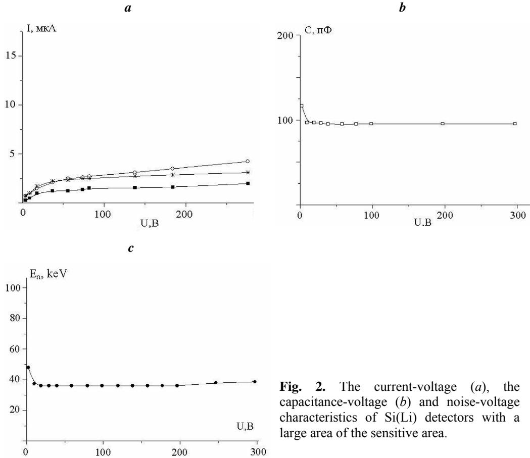
**Fig. 2.** The current-voltage (a), the capacitance-voltage (b) and noise-voltage characteristics of Si(Li) detectors with a large area of the sensitive area.
