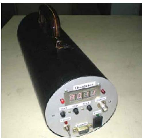
**Fig. 4.** The appearance of Radon radiometer.
