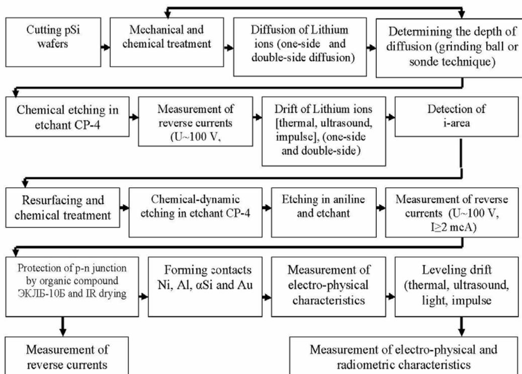
**Fig. 1.** Technological route of the development of Si (Li) detectors.
